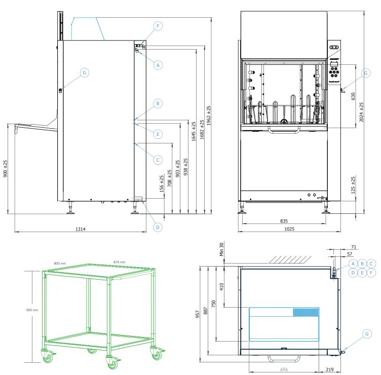
EcoExchanger® unit (optional add-on). The EcoExchanger unit (heat recovery and steam reduction) must be connected to a cold water feed at all times.(F) Note: EcoExchanger is only available for cold water option machines (max power 32A, 16,5 kW) but on site, the machine can be connected to either a hot or a cold water feed. (A)
